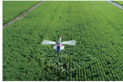
Aerial agricultural spraying using unmanned helicopter
